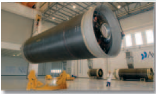
The P80 motor case (length 10 m, diameter 3 m) at Avio in Colleferro (I). The case is then shipped to French Guiana for propellant casting, integration of components such as the nozzle, thrust vector control and sensors. The qualification firing is scheduled for November 2006 on the site's BEAP test stand. (ESA/S. Corvaja)
