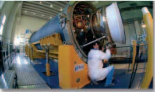
The Z23 Zefiro stage-2 solid-propellant motor is prepared for shipment to Sardinia for the June 2006 firing test.
