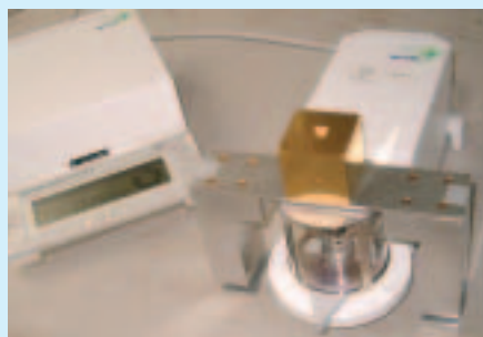
The LISA Pathfinder Engineering Model proof-mass undergoing magnetic susceptibility testing at the International Bureau of Weights and Measures (BIPM) in Paris
