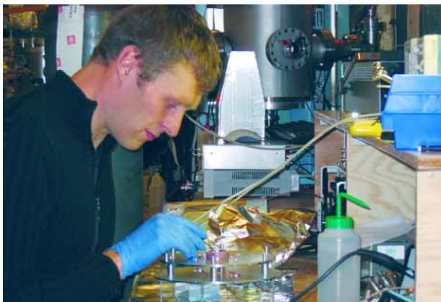
The procedure working on the LAMA instrument required some laboratory experience. Here, Markus Landgraf works on the sensitive micro-channel plate, which is at the heart of LAMA's ion detector electronics
