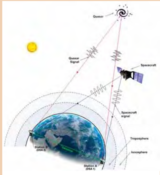
Delta-DOR tracking of a deep-space probe and of a nearby quasar from DSA-1 (New Norcia, Australia) and DSA-2 (Cebros, Spain). The effects of common error sources between spacecraft and quasar observations are cancelled by the quasar tracking.
