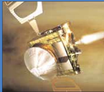
Artist's impression of Venus Express during the Venus orbit insertion manoeuvre on 11 April 2006. The spacecraft's main engine burned for about 50 minutes, to reduce its speed with respect to Venus to allow the the spacecraft to be captured by the planet's gravitation (ESA/AOES Medialab)
