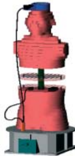
Matroshka consists of 25 mm-thick slices.
