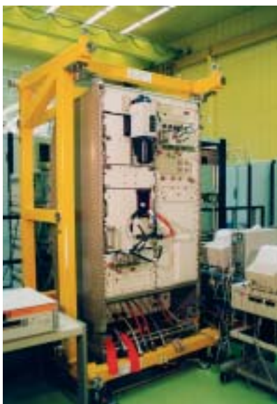
The Fluid Science Laboratory undergoes testing in the RLTF.
