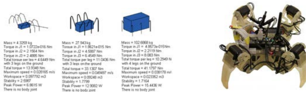
Figure 1: Left: Evolved morphologies under different task descriptions, from [9]. Right: Robot used for evolving walking gaits in [10].
