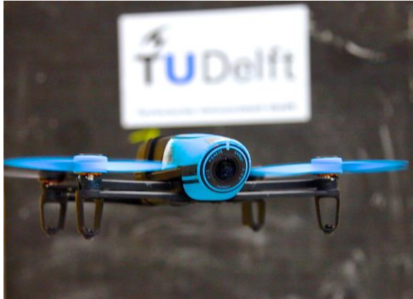
Fig. 6. A Parrot Bebop 1 is used as the flying platform. The original autopilot is fully replaced by an open-source autopilot called Paparazzi UAV.
