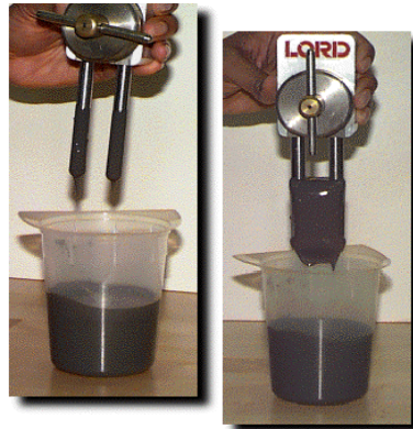
Figure 2.1: Rheological behaviour of a MR fluid (from[9]).
