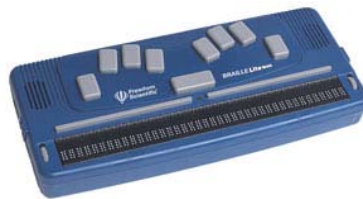
Figure 3.3: Examples of refreshable Braille display based on piezoelectric actuators (from [15]).
