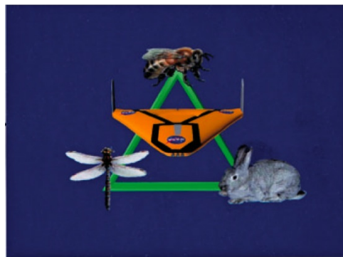
Figure 3.3: The concept of incorporating best of class capabilities to develop a hybrid flyer taking inspiration from insects (honeybees and dragonflies) for autonomous navigation algorithms and from mammals (rabbits) for object recognition and tracking. From [Thakoor, 2003].
