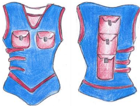
Figure 2 Example of a garment model without sleeves, with side closure made by velcro straps and with pockets designed to accommodate the shielding materials, for IVA (Intra Vehicular Activity).
