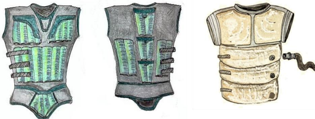
Figure 3 Examples of possible garment models for EVA (Extra Vehicular Activity). On the left and in the center: garment padded with rigid bars or gel pockets(front and back). On the right: inflatable garment fillable with water or gel.
