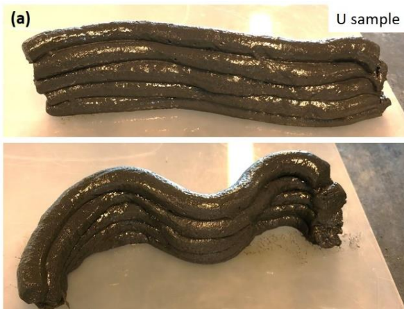
Figure 12. Layer-by-layer buildability of (a) mixture containing 3% urea (U sample), (b) mixture containing 3% naphthalene-based admixture (N sample).
