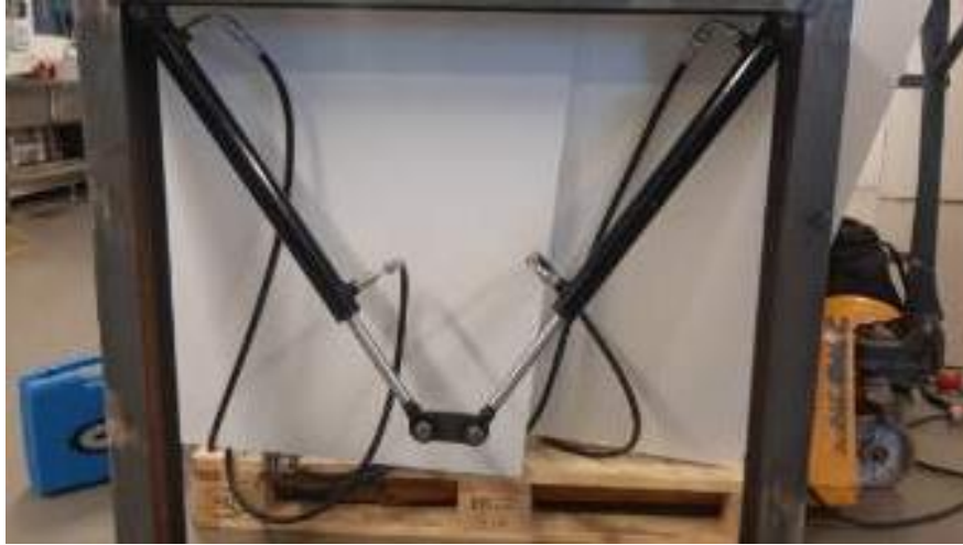
Figure 8. Internal view of the chamber frame with two pneumatic actuators visible.
