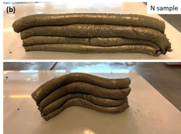
Figure 12. Layer-by-layer buildability of (a) mixture containing 3% urea (U sample), (b) mixture containing 3% naphthalene-based admixture (N sample).
