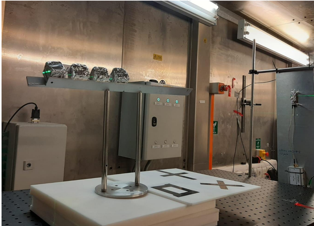
Figure 5. Experimental setup for ChipIR experiments. Four samples are arranged in a dedicated sample holder, courtesy of A. Meurisse. The green laser light indicates the path of the neutron beam. Detectors to measure transmission are placed before (not shown) and after (visible on the right-hand side panel) the samples.
