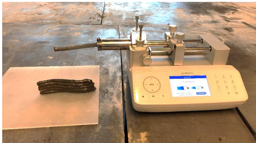
Figure 4. A high-pressure syringe pump is utilized for 3D-printing the samples.
