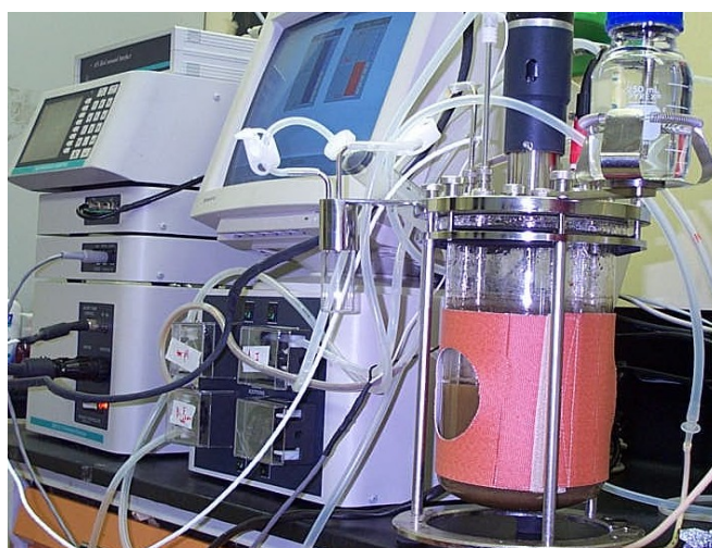
Figure 8-1. Two tank bioreactor system to produce hydrogen.
