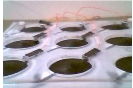
Fig. 4 Array of dielectric active polymer actuators. [16]
