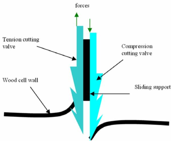
**Fig. 4:** Simplified model of ovipositor drill [28].
