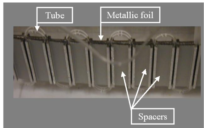
Fig. 1: Prototype of the spider inspired actuator [11].
