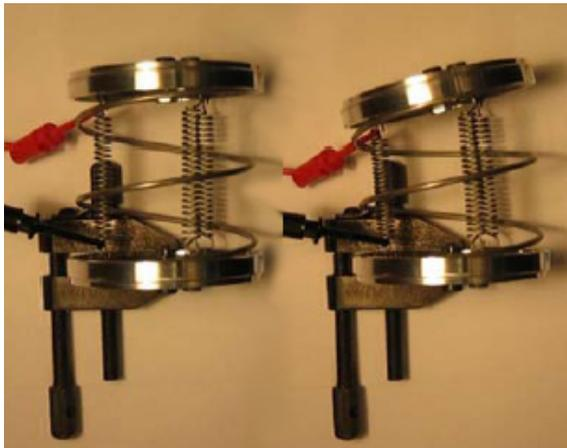
**Fig. 2:** Experimental set-up of a mechatronic joint before (left) and after one of the internal SMA springs was heated with a 2 A current (right) [12].
