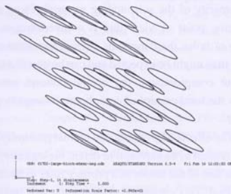
Fig. 13 Magnified view of the deformed and undeformed holes under negative shear.
