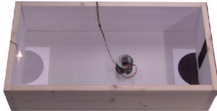
Figure 163 – Bird's-eye view of the light switching arena. The Khepera switches on the light if it passes over the black area and gains fitness by staying in the grey area while the light is on. The robot can detect ambient light and the colour of the wall but not the colour of the floor.
