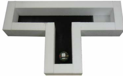
Figure 168 – Experimental set up for testing transfer of the controller to a real Khepera robot
