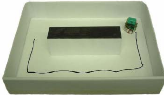
Figure 156 – The testing arena for the Alice robot. The trajectory is the distance covered in 10 seconds overlaid from video footage. The arena is 25 x 18cm.
