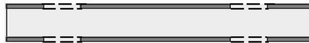
(a) Shallow boron diffusion to define beams, proofmass, and supporting rim. Nitride deposition and definition for electrode anchors and isolation dielectric underneath electrode dimples.
