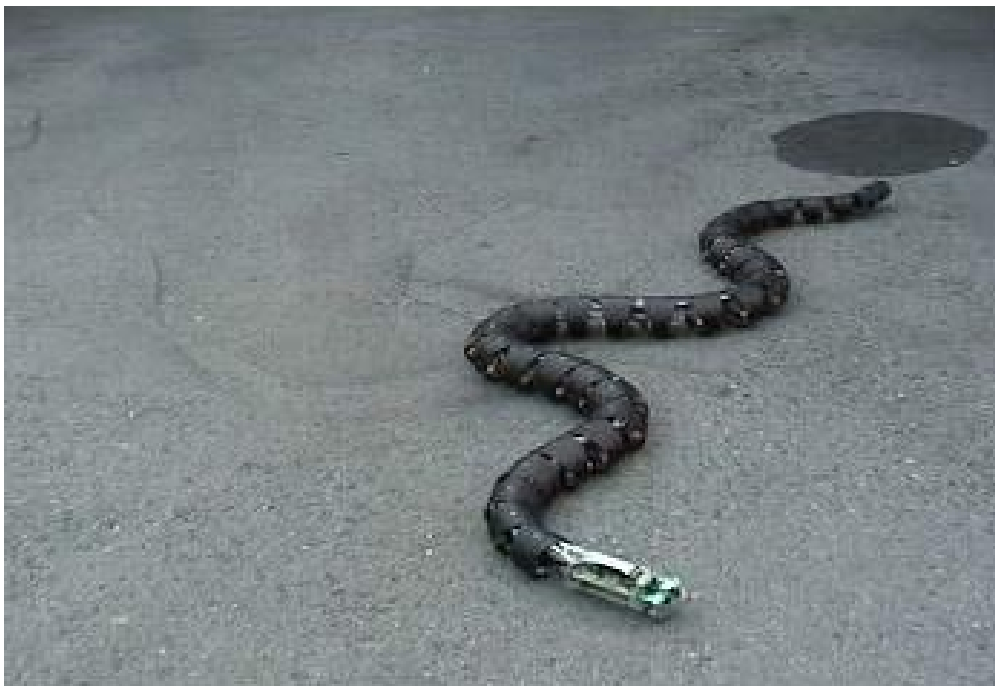
Figure 3.10 – a snake robot employing horizontal undulation to move
