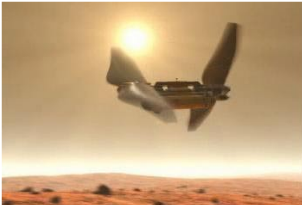
Figure 3.8 – conceptual image of the entomopter flying across the surface of Mars. Note the two seesaw wings operating out of phase.
