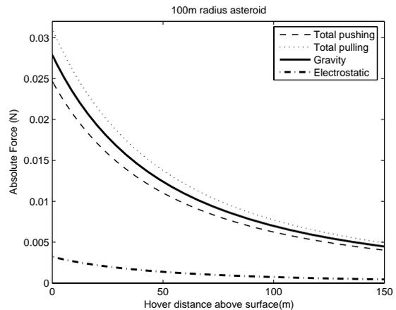
Figure 11: 100 m asteroid radius. Both asteroid and spacecraft charged to  $20kV$
