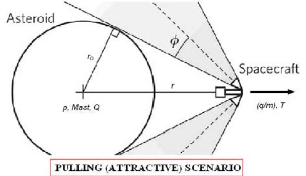
Figure 4: Spacecraft and asteroid are charged to opposite polarities. Figure adapted from [7]. The engines need to be canted.
