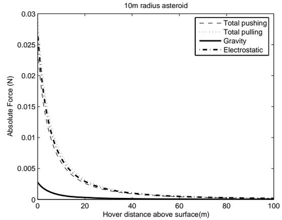
Figure 13: 10 m asteroid radius. Both asteroid and spacecraft charged to 20kV
