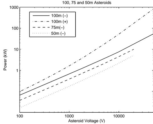
Figure 7: Total power required to maintain different sized asteroids at a given voltage. Negatively charged asteroids are mainly considered as this is more efficient.
