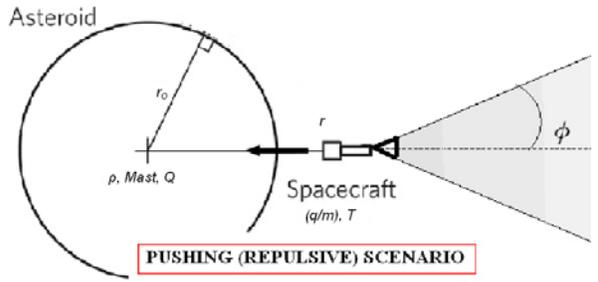
Figure 5: Spacecraft and asteroid are charged to the same polarity. Figure adapted from [7]. The engines do not need to be canted.
