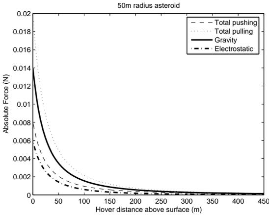
Figure 12: 50 m asteroid radius. Both asteroid and spacecraft charged to 20kV
