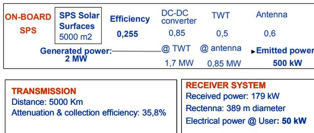
Figure 9: Performances of RF based SPS
