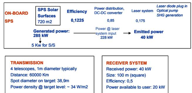
Figure 10: Performances of laser based SPS
