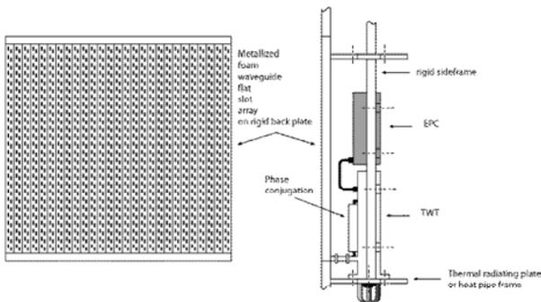
**Figure 7:** On board slot array antenna technology
