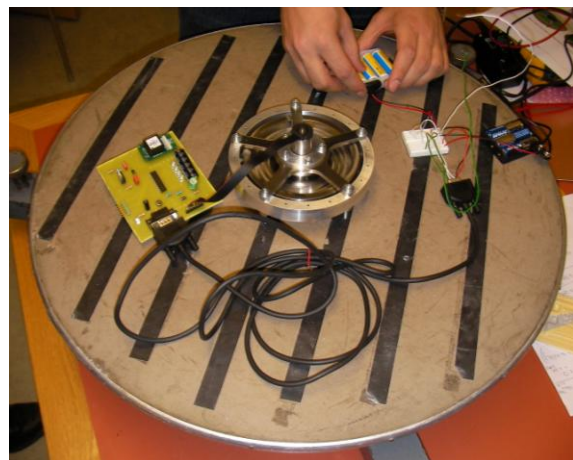
Fig. 6. Flight version of reaction wheel assembly tested on low friction rotating platform.
