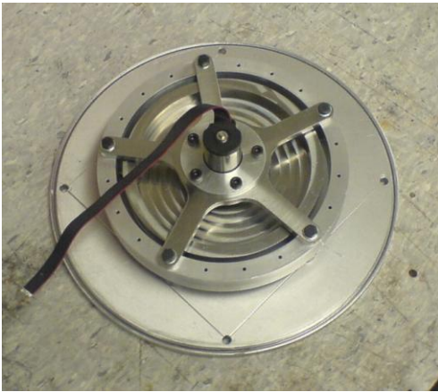
Fig. 7. Manufactured reaction wheel assembly.
