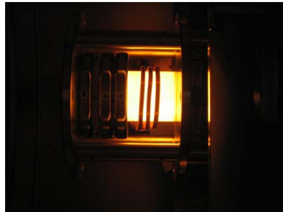
Figure 10. DS4G laboratory prototype thruster pictures with Xenon RF discharge at 400 W power during thermal testing (no high voltage feedthroughs present)
