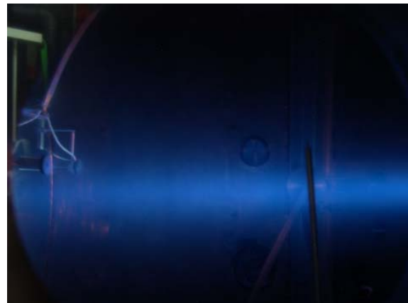
Figure 11. The DS4G beam inside the vacuum chamber and the dedicated diagnostics
