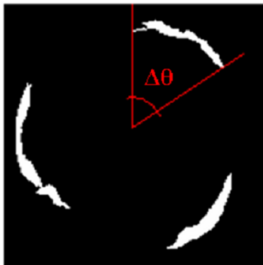
Figure 13. Evaluation of the azimuthal extension of the cavitation on a blade.
