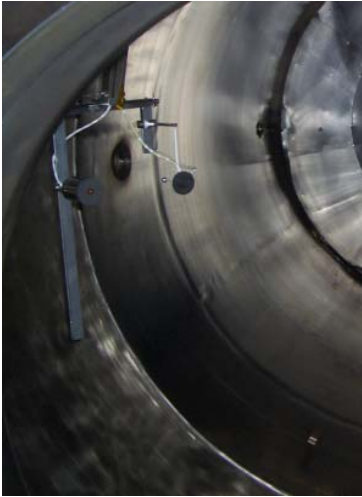
Figure 7. Calorimeter and Langmuir probe mounted in CORONA test facility.
