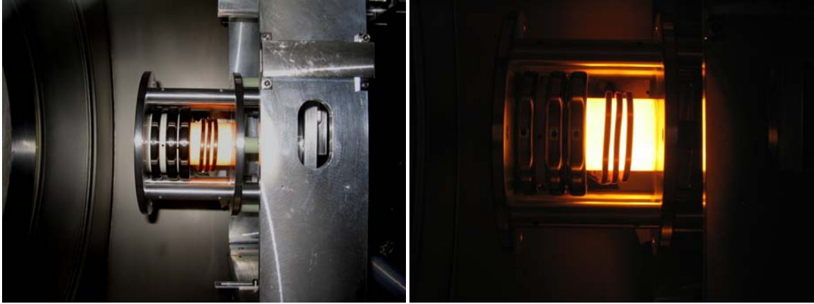
Figure 9. DS4G laboratory prototype thruster with Xenon RF discharge at 400 W power during thermal testing (no high voltage feedthroughs present)
