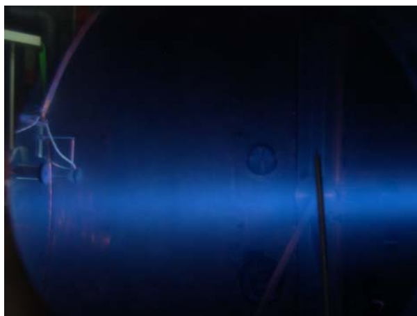
Figure 10. The DS4G beam inside the vacuum chamber and the dedicated diagnostics
