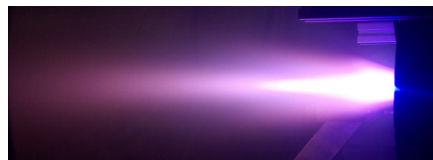
Figure 1: Plume of the AF-MPD ZT1 thruster in steady-state operation with 5.4 kW (Argon)
