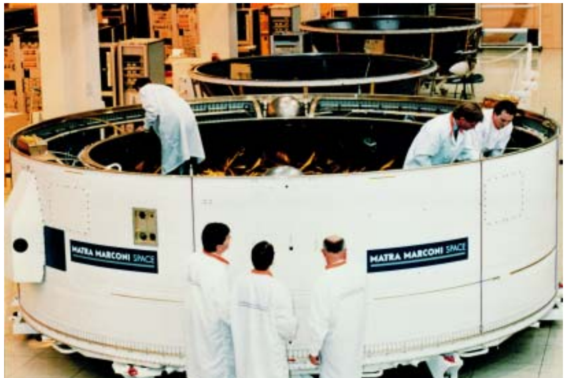
Ariane-5's Vehicle Equipment Bay (VEB) carries the control systems. Stage-2 sits on the inner truncated cone.
