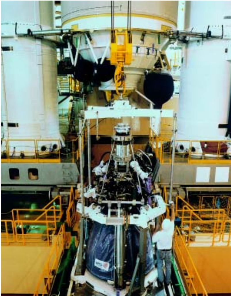
Preparing to install the Vulcain main engine on Ariane-5. (ESA/CNES/CSG)
