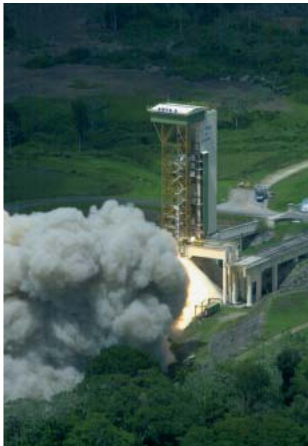
The 125 second booster static firing in progress on the BEAP test stand in Kourou
