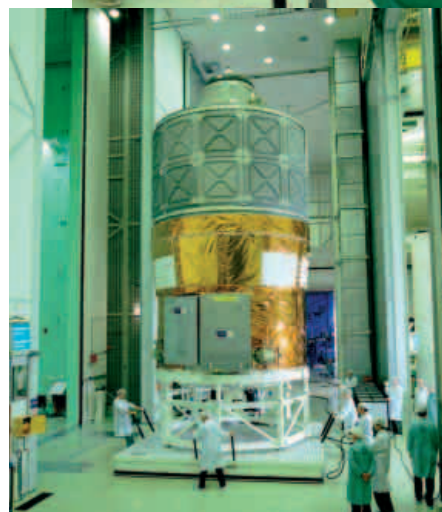
The ATV structural-thermal model in the ESTEC Test Centre
