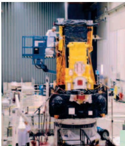
Integral undergoing sine-vibration testing in the ESTEC Test Centre
