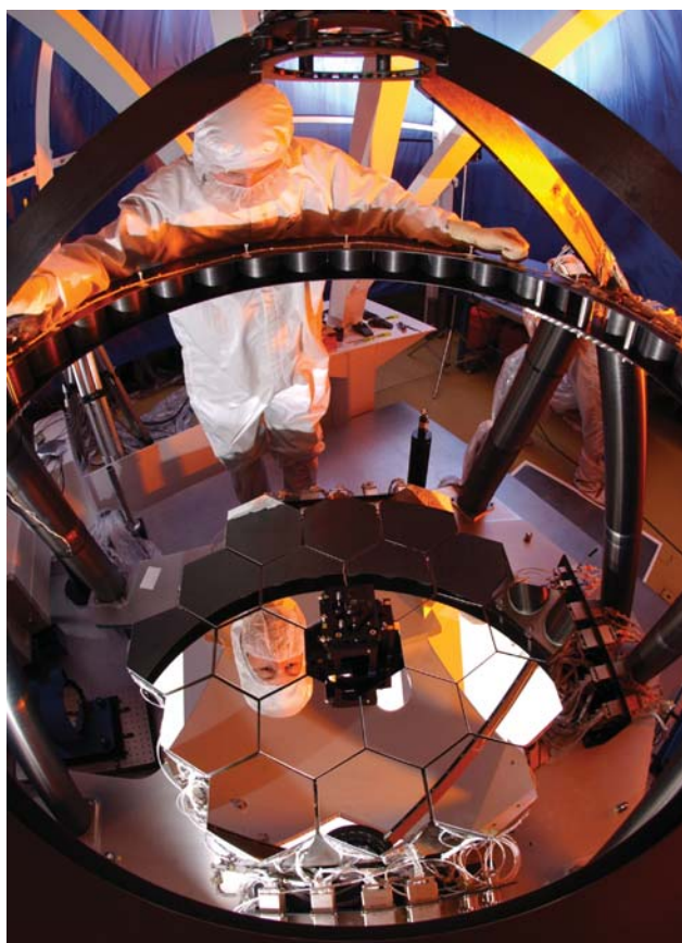
JWST wavefront sensing and control testbed to demonstrate the feasibility of the active alignment approach for the main telescope. The testbed is a scaled-down model of the full telescope, including actuators
