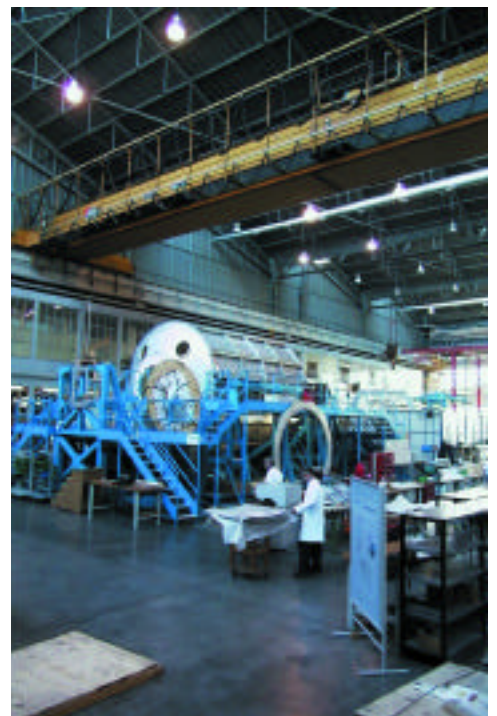
Columbus Module flight-unit primary structure in fully welded configuration, at Alenia in Turin (I)
