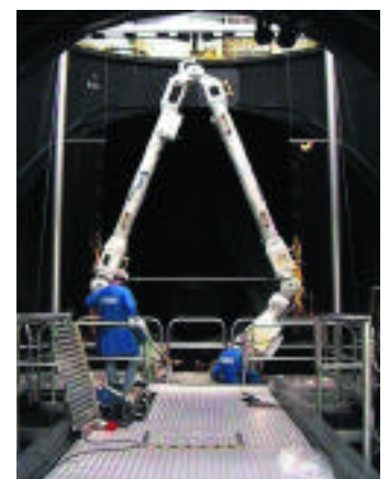
Installation of the ERA engineering qualification model in the Large Space Simulator (LSS) at ESTEC (NL), for heat-balance testing
