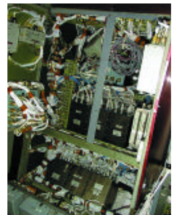
DMS-R Fault-Tolerant Computers installed in the Russian Service Module
