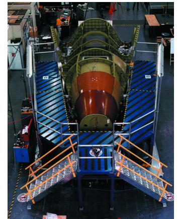
The V201 space-test X38 prototype under assembly at NASA's Johnson Space Center
