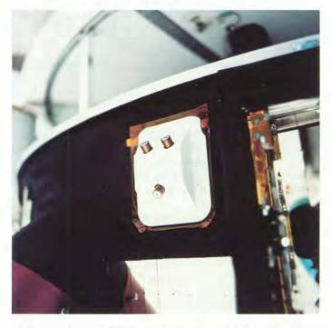
Epona on the experimenters' platform - flight model of the Giotto spacecraft. The three telescopes are very clearly seen.
