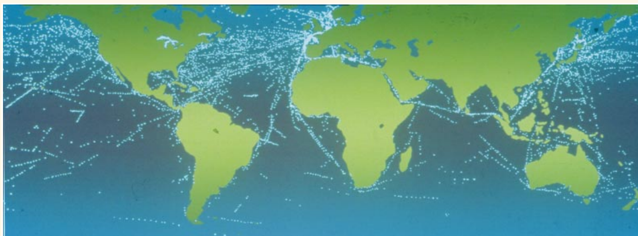
Wind measurements made by ships and satellites. Above: Ship in-situ wind measurements for the three-day period 31 October - 3 November 1990, each dot representing one wind-speed/direction report. Below: One day of ERS-1 Wind Scatterometer measurements in March 1992
