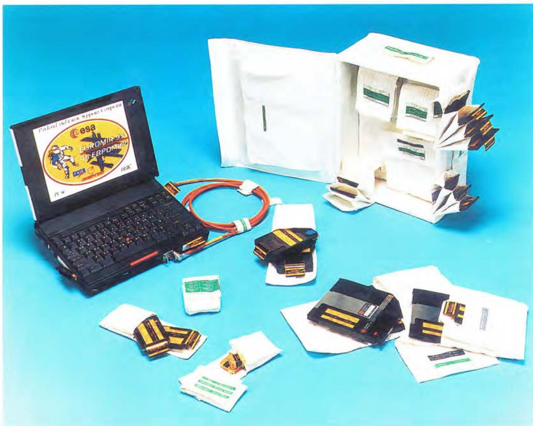
Figure 4. The Payload and Crew Support Computer (PCSC), accessories and peripherals with the onboard stowage bag
