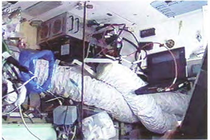
Figure 6. Laptop connected to the Mir Interface Payloads System (MIPS) during telemetry transmission
