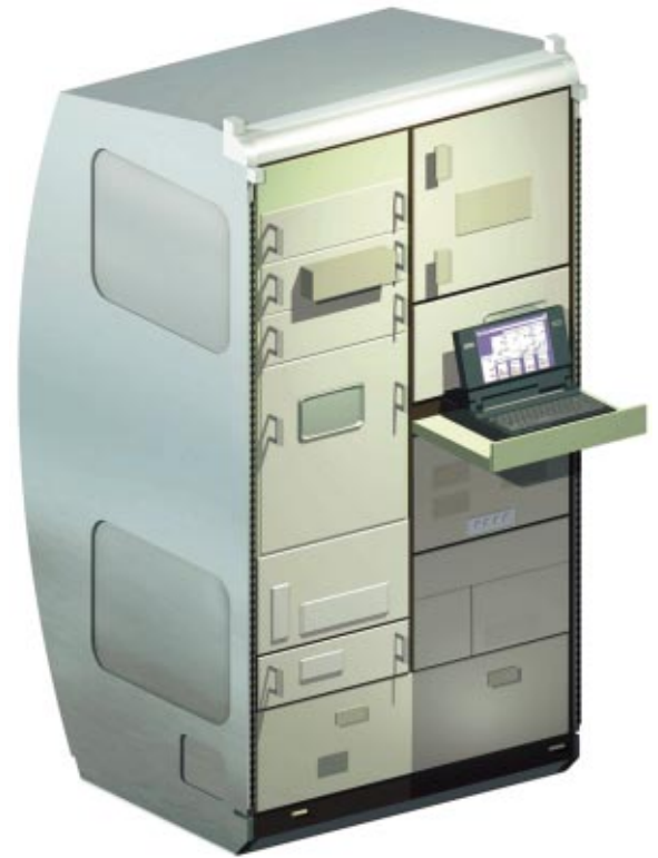
Fig. 29. The Fluid Science Laboratory will study fluid behaviour in the absence of gravitational effects. (ESA/D. Ducros)
