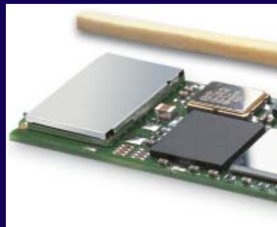
This Ericsson Bluetooth module is extremely compact
