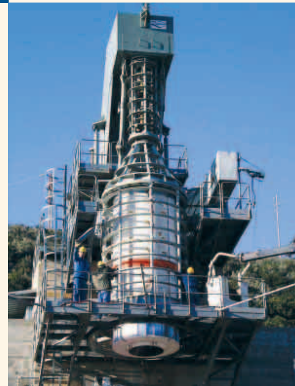
Preparation of the Zefiro 16 qualification-model motor for test firing at the Salto di Quirra test range in Sardinia, Italy
