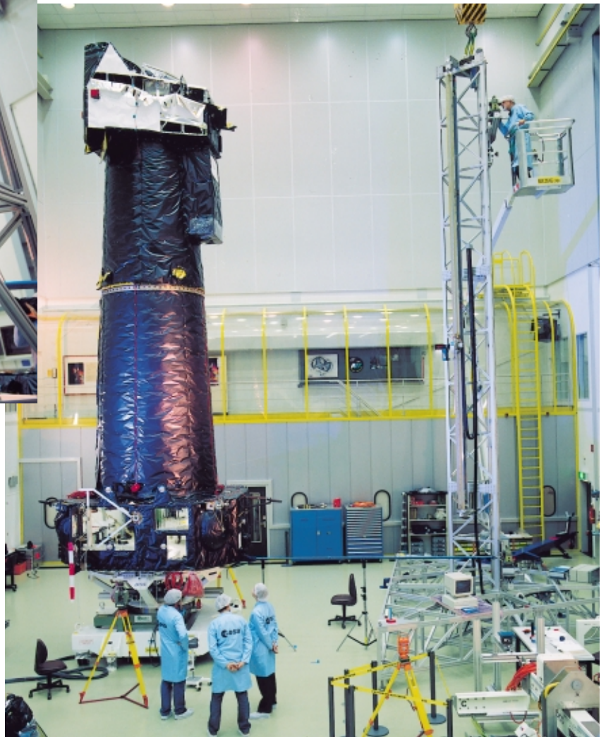
Figure 5. The STM XMM spacecraft assembled on the alignment rotary table. The alignment stand is on the right
