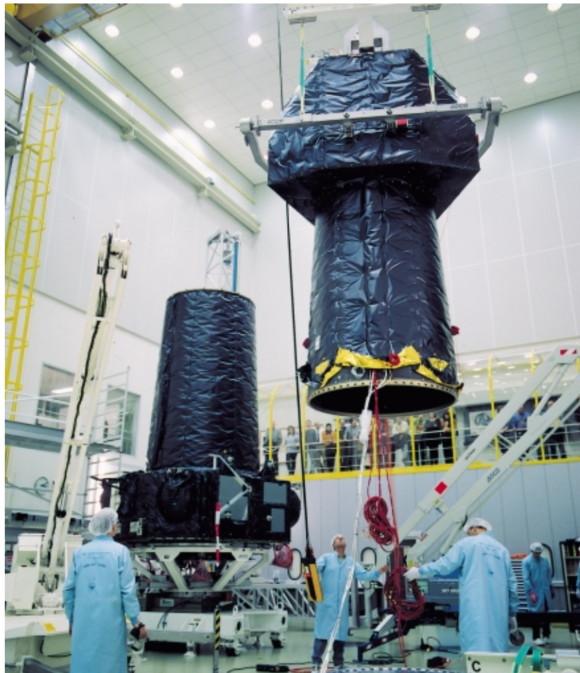
Figure 2. The XMM STM Lower Module (left) and Upper Module (right) at ESTEC
