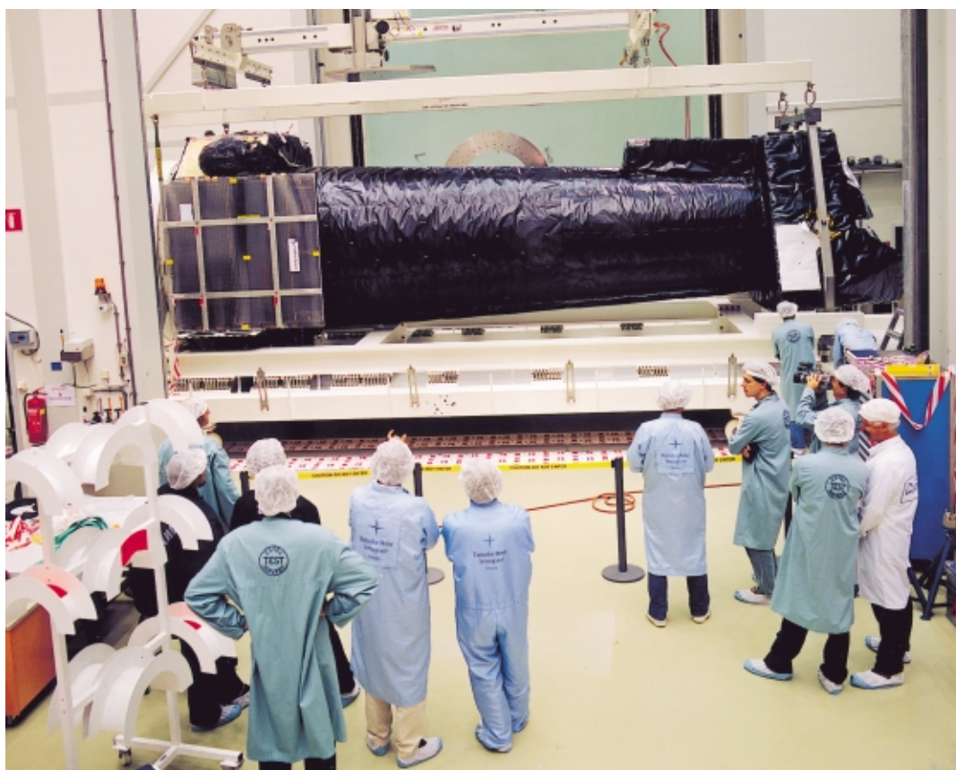
Figure 7. The XMM PFM spacecraft assembled and attached to the container chassis before closure of the container lid
