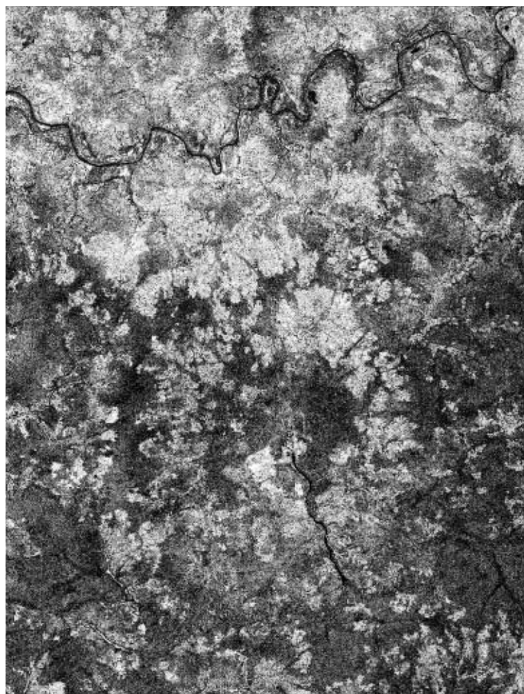
Figure 4. Coherence image (phase correlation between the two acquisitions) computed from an ERS tandem pair of SAR images, taken on 23 and 24 December 1995. Bright areas represent high coherence, which include scarce vegetation and settlements. Dense vegetation is less coherent and appears darker, while water always appears black (no coherence). Coherence images are also useful for DEM quality assessment and for change detection
