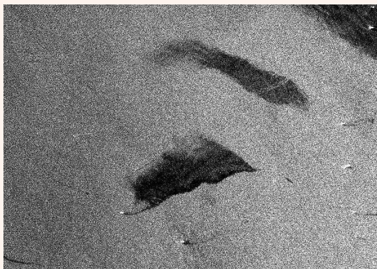
Figure 2. ERS-2 SAR scene acquired on 18 July 1996 showing oil slicks in the North Sea
