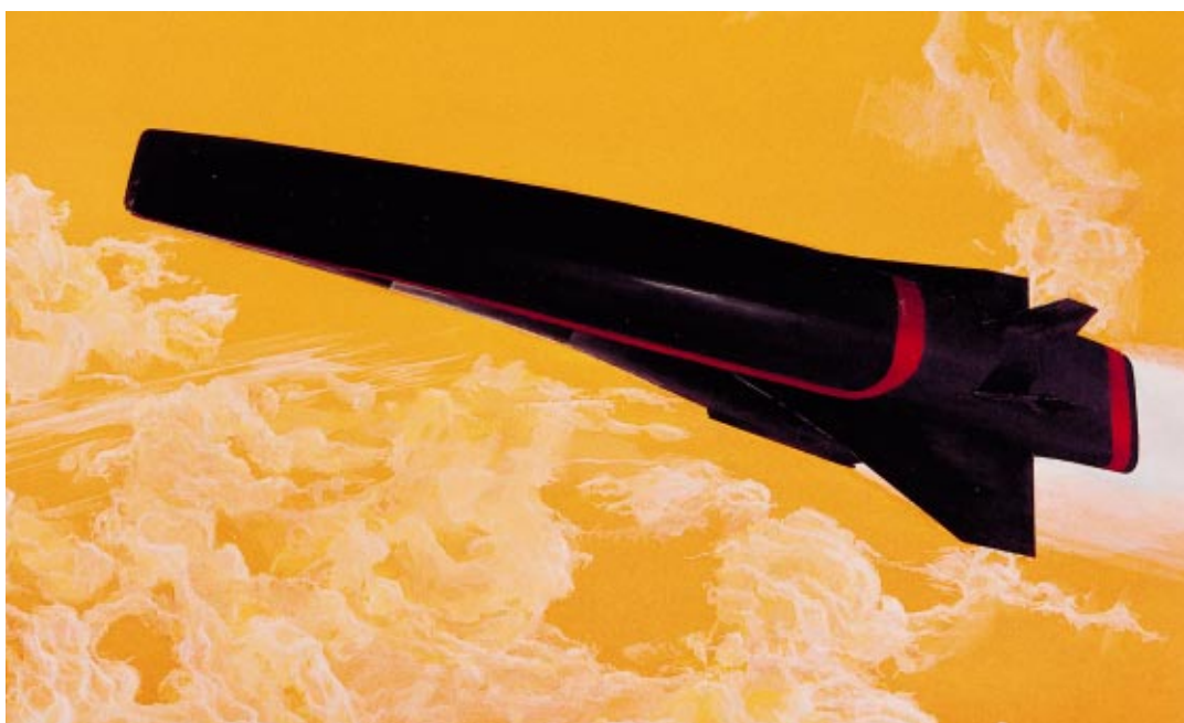
Figure 4. An ESA Winged Launcher Configuration (WLC) studied, by DASA leading a team of European companies, in the late 1980s. It has a supersonic combustion ramjet air-breathing propulsion system (courtesy of British Aerospace)
