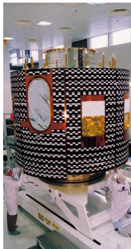
MSG-1 structural and thermal model during integration at Aérospatiale in Cannes (F)
