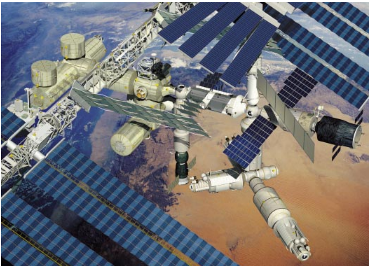
Figure 2. Docked to the Russian Service Module, the ATV is capable of reboosting the ISS into a higher orbit (ESA/D. Ducros)
