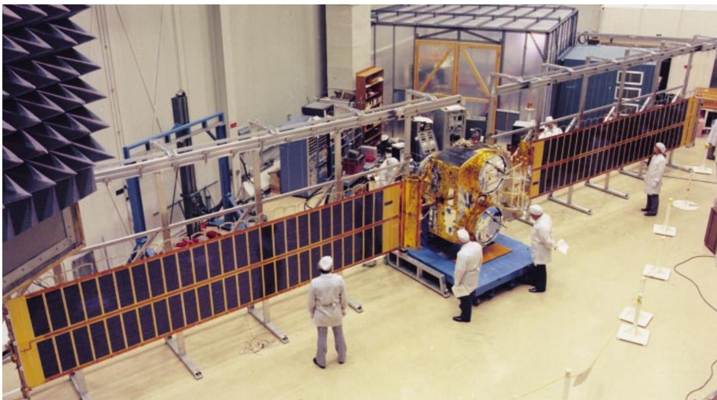
Figure 5. CTS-Hermes engineers monitoring solar-array deployment in the high bay of the David Florida Laboratory, near Ottawa (photo courtesy of Communications Research Centre)
