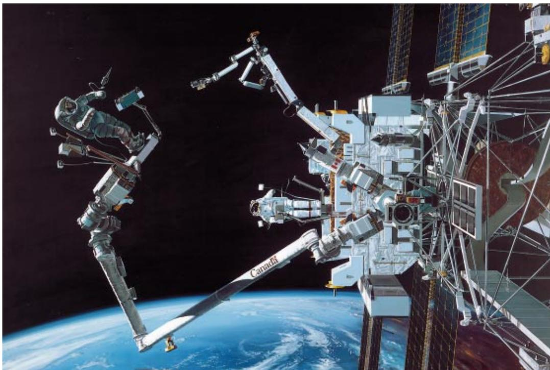
Figure 4. Canada's contribution to the International Space Station, the Mobile Servicing System that will be essential in the assembly, maintenance and servicing of the ISS (photo courtesy of CSA)
