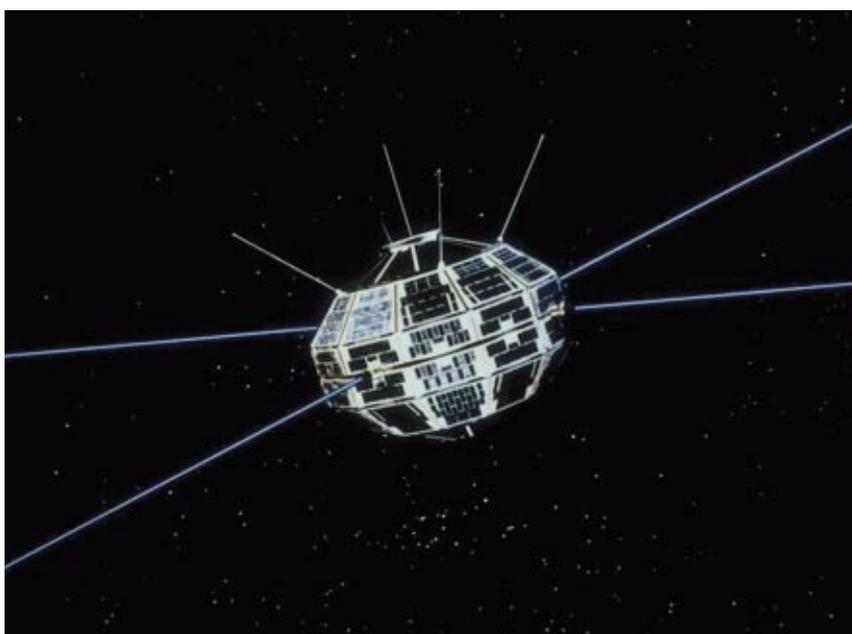
Figure 1. Alouette-1, Canada's first research satellite for the study of the ionosphere (photo courtesy of CSA)
