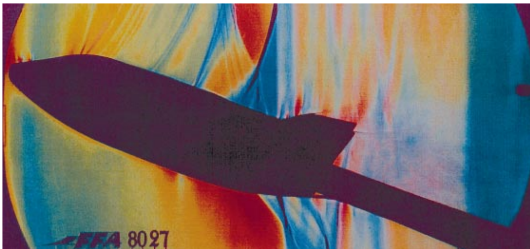
Figure 4. Schlieren photograph of an X38 flow field during testing at FFA in Sweden
