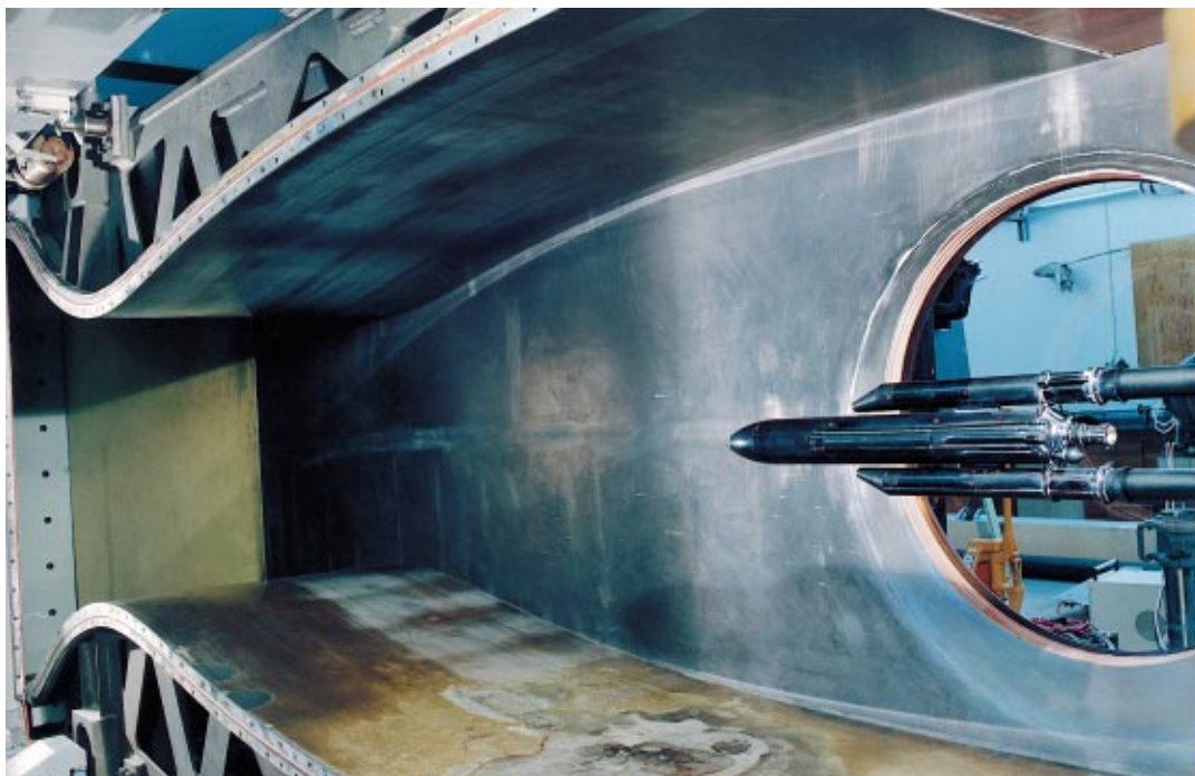
Figure 10. Ariane-5 model for buffeting studies at FFA in Sweden
