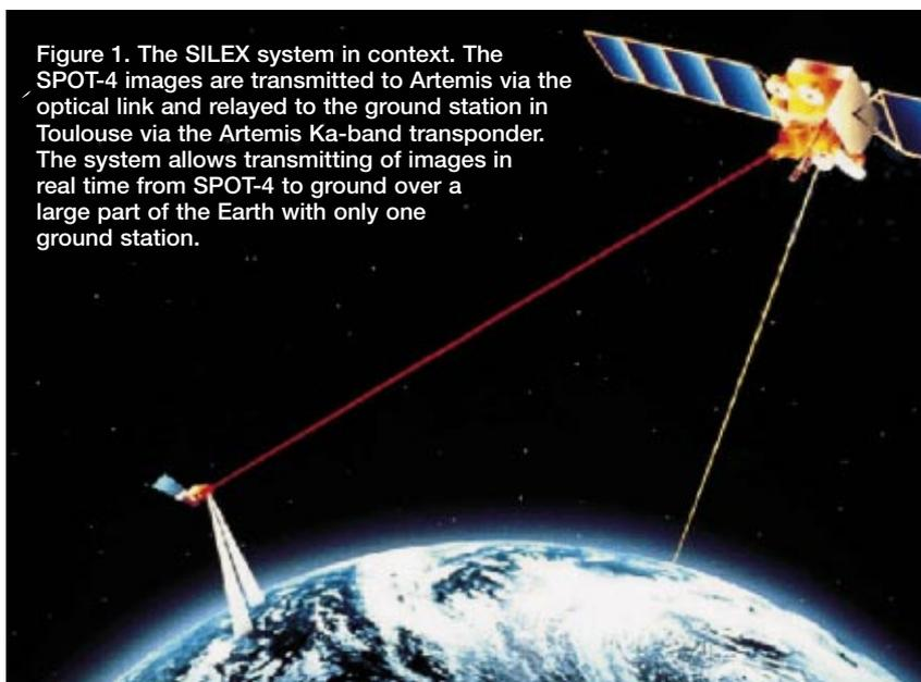
Figure 1. The SILEX system in context. The SPOT-4 images are transmitted to Artemis via the optical link and relayed to the ground station in Toulouse via the Artemis Ka-band transponder. The system allows transmitting of images in real time from SPOT-4 to ground over a large part of the Earth with only one ground station.
