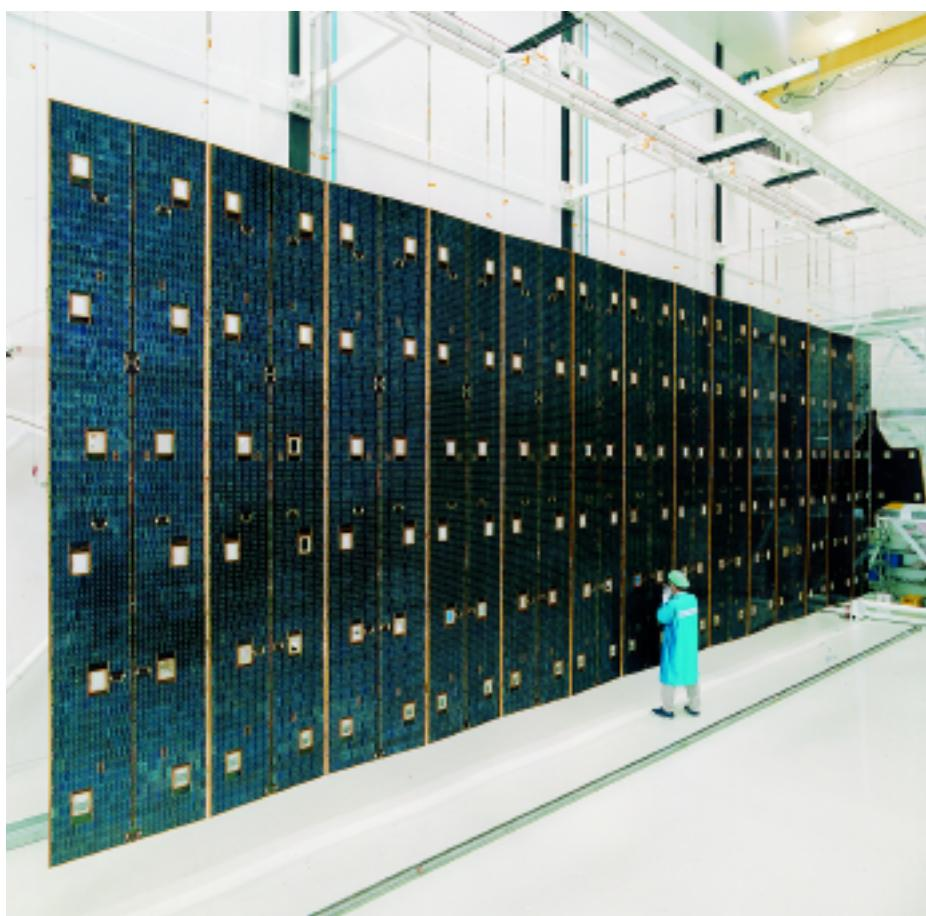
Envisat/Polar Platform flight-model solar-array deployment during acceptance testing at Fokker Space (NL)
