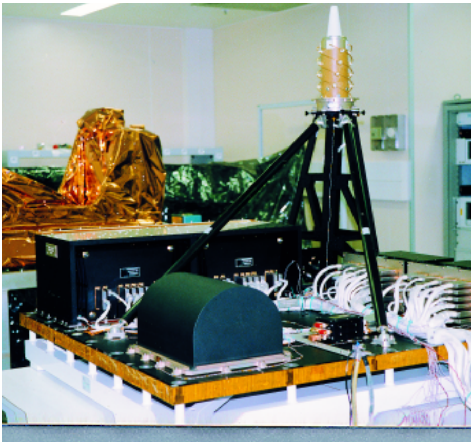
Flight model of the Envisat DORIS/MWR instrument composite undergoing final testing prior to delivery to Matra Marconi Space (B)
