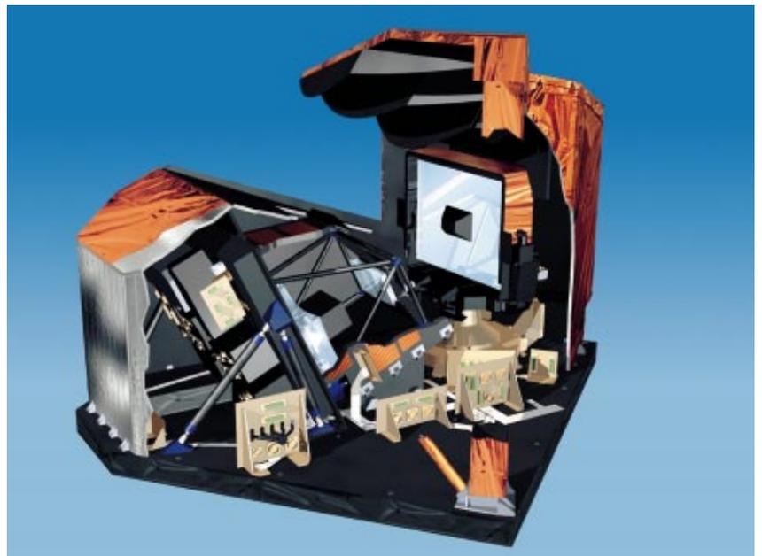
Figure 3. Cut-away drawing of GOMOS
