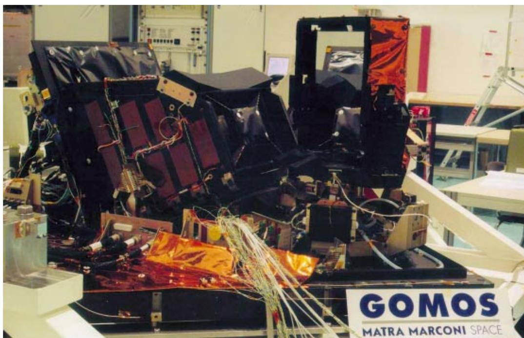
Figure 4. GOMOS telescope assembly during integration at Matra Marconi Space, in Toulouse (F)
